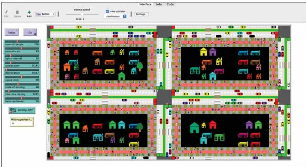
Figure-3: NetLogo control panel and graphics window showing parameter sliders on the left and the simulated 2-D traffic scene on the right.
