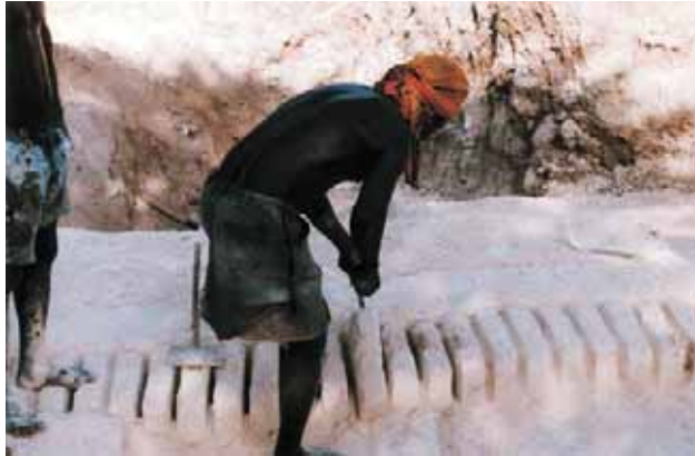
Figure-5: Workers and coral lime stones mining techniques in Manda Island, Lamu archipelago, Kenya Source: S. Pradines
