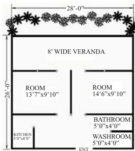
Figure-5: Original plan of F-Type barrack given to the Federal Employees consisted of, a verandah, two rooms, common bathroom, washroom and kitchen, and also a provision of back alley Source: Drawn by Author after visiting the houses.
