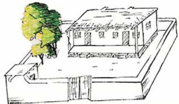
Figure-36: Courtyard with Trees to Increase Level of Humidity
