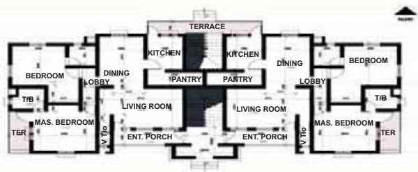
Figure-6: (Type 3) Typical Ground Floor Plan of Two Families' Semidetached Storey Housing Unit in the Study Area.
