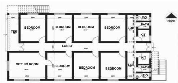
Figure-12: (Type 7) Typical Ground Floor Plan of a Single Storey Tenement Housing in the Study Area.
