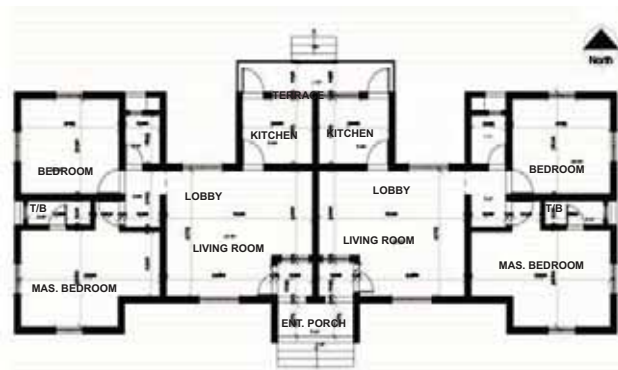
Figure-10: (Type 5) Typical Ground Floor Plan of Two Families' Semidetached Bungalow Housing Unit in the Study Area.
