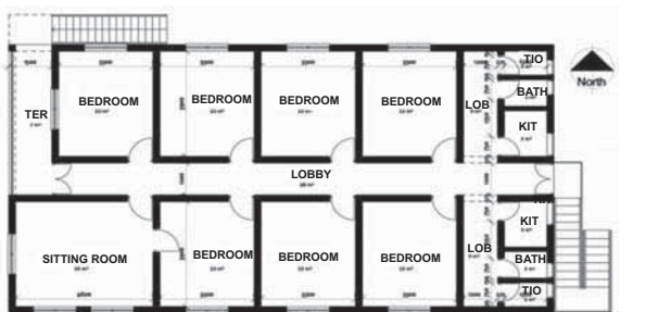
Figure-13: (Type 7) Typical First Floor Plan of a Single Storey Tenement Housing in the Study Area.
