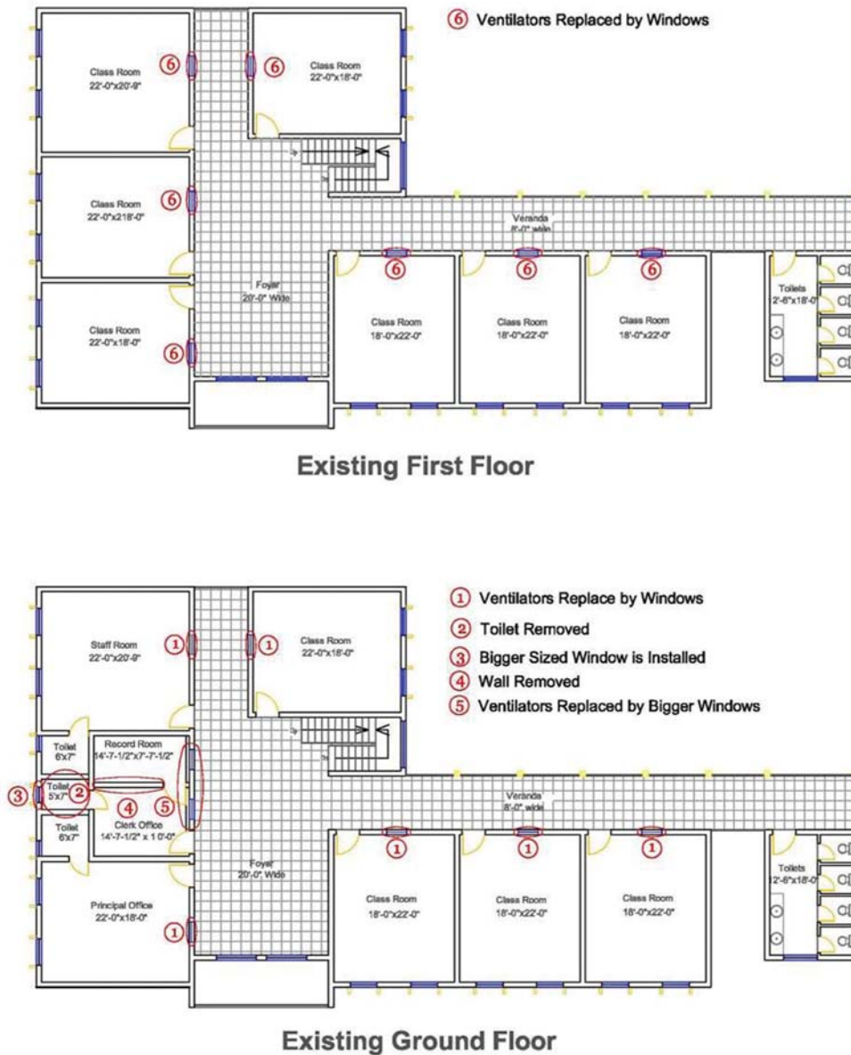
Figure-16: Alterations Proposed in Existing Building Plan.
