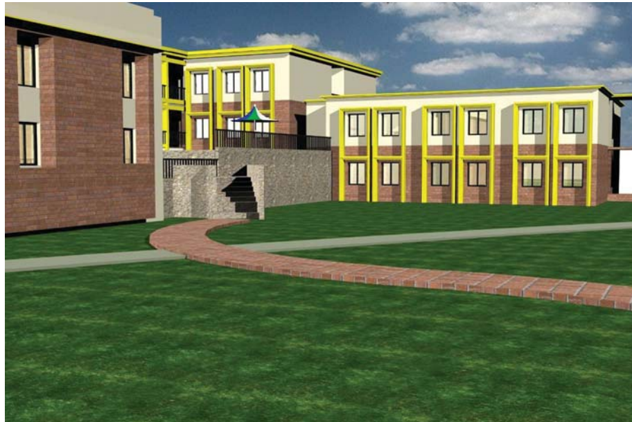
Figure-23: Locally available red bricks on exterior walls.
