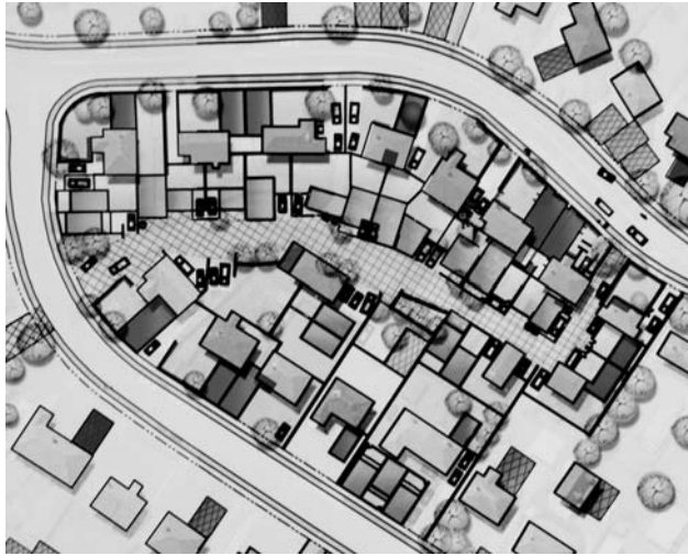
Figure-4: Site plan proposal by Entry No 3. The central driveway is the only form of common open space in the scheme and is poorly developed for people.
