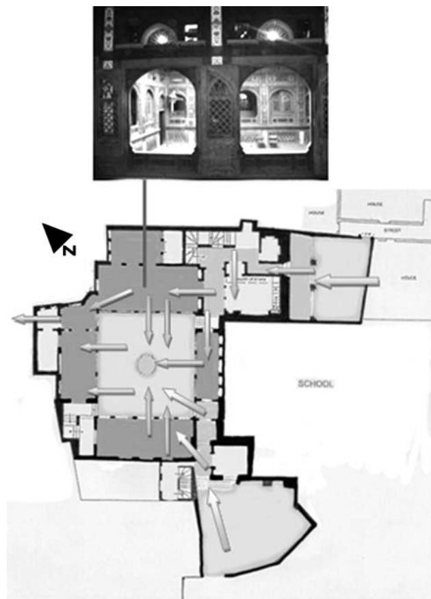
Figure-5: Orientation of the rooms to the prevailing breeze, and the exchange of hot and cool air.
