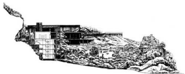
Fig-32: Sectional elevation of the Kandalama Hotel designed by Geoffrey Bawa in Dambulla, Sri Lanka built between 1991-94. This elevation shows the relationship of the building to the cliff. It was designed not so much as a building to look at but a building to enjoy the views from. (Bawa Archive)
