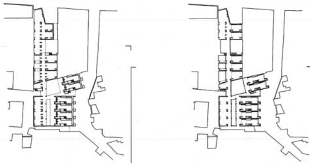
Figure 36 : Ground Floor and First Floor Plans of Community Housing.
