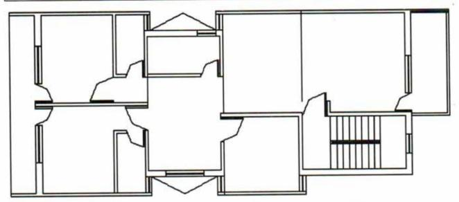
pipes to the toilets and kitchen in the previous proposal, toilets were in both sides, so the required length of service pipes was much more. Here they were at one side and when two adjacent houses are arranged in a mirror image, the cost again reduces to half. One toilet is reduced in size but the other developments are significant. Moreover the cost has again been reduced considerably. (See bar diagram)
